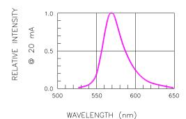
Fig.5 RELATIVE INTENSITY VS. WAVELENGTH
