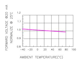
Fig.3 FORWARD VOLTAGE VS. TEMPERATURE
