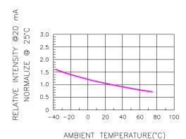
Fig.4 RELATIVE INTENSITY VS. TEMPERATURE
